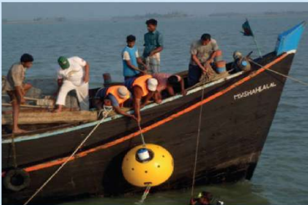
ADCP being deployed on the seabed
